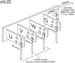
Figure 22. UVWO Terminal Lugs 3Ø-240V Connections
